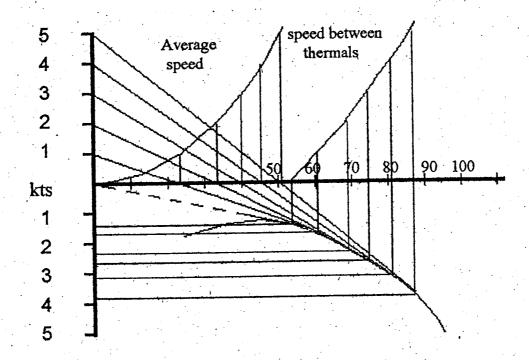
These curves represent the optimum speed to fly between thermals, and the average speed that will result from their application. It is often useful to have these speeds tabulated for use in flight planning as well.
