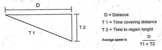
The performance curve of a sailplane provides the basic information for the McCready system of flying. Each type has its own performance curve, McCready speeds to fly and resultant average speeds.
