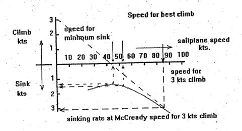
By drawing tangents to the curve form above the zero, the speed to use between thermals may be found at the point of contact between the tangent and the curve. The average speed which results from the application of this system will be given by the intersection of the tangent and the axis of the graph.
